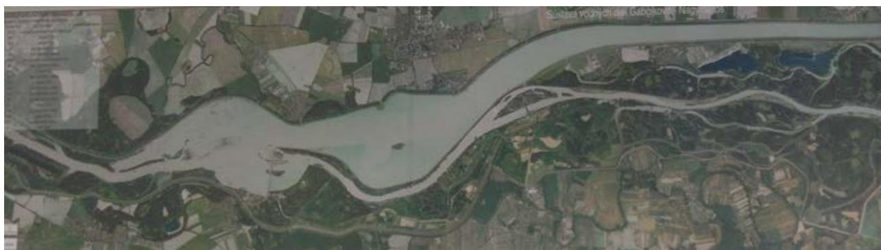
Figure 2. A photo of the man-made canal - 40km - and the natural riverbed of the Danube river in the area of the water scheme 136
